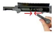
7. To confirm correct assembly, press the back of the firing pin several times through the bolt tube window. The pin should pass through the bolt face smoothly and easily and retract quickly. If you encounter any problems, after reattempting assembly, please contact us.
