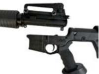
2. Using a 3/32" punch, remove the bolt catch roll pin. Suggestion: place durable tape on the surface of the lower receiver to help prevent scratching the finish.
