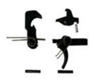
The Big Kahuna Heavy Duty Hammer & Spring (included with your upper) will be inserted, oriented as shown. Dont install until step 5.
