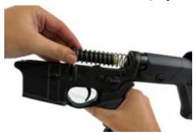
8. Remove the buffer retention pin and spring. To remove these parts, you will need to unscrew the buffer tube. Important: this step releases pressure on the takedown pin detent and spring. Remove the stock very slowly and be careful not to lose control of the detent and spring or else they will shoot across the room.
