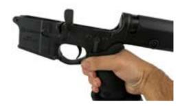
6. Optional: Using a pair of needle nose pliers, install the E-clips on the hammer and trigger anti-walk retention pins. Suggestion: insert the pins so that the undercut is flush with the receiver, lay the pin flat on the receiver and squeeze the clips gently into place. Use caution to avoid scratching the lower receiver finish.
