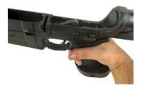
7. Remove the buffer and buffer spring. To do this, depress the buffer retention pin. Note: the buffer is spring loaded and will jump free as the retention pin is depressed. Slide and remove the buffer and buffer spring from the buffer tube.
